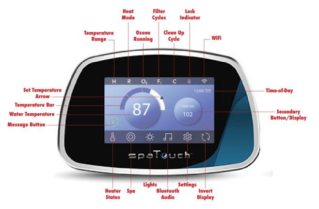
When the spa is powered On, four dashes appear in the Water Temperature display for one minute. The dashes indicate that the spa is checking the water temperature. After the pump runs for 1 minute, the dashes disappear and the water temperature is displayed (B). The dashes may reappear after the pump has not run for one hour.
