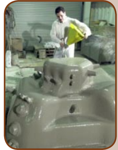
The acryment is applied to the back of the Lucite Acrylic Shell acting as a heat sink, which draws the UV and heat into this sub surface dispersing it evenly, instead of damaging the surface of the acrylic. The Acryment eliminates the uneven expansion and contraction associated with fiberglass backed shells that are known for there blistering and cracking. This acryment re-enforcement process is unique to Wind River Spas.
